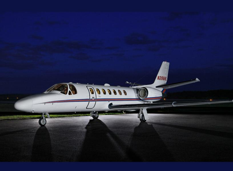
The Encore offers a range of 1,800 nmi with seating up to 8 passengers.
